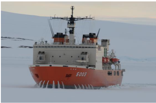
12,500ton,138 x 28 x 16m,179 crew, Members observe 80 Fig.1 The new icebreaker "Shirase".
