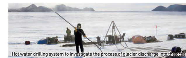
Hot water drilling system to investigate the process of glacier discharge into the ocean
