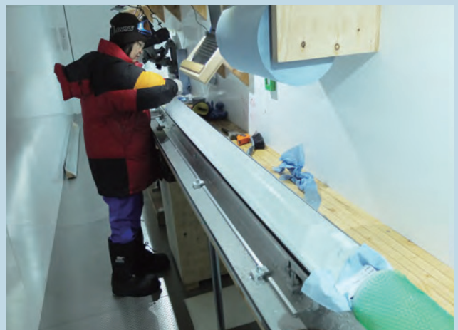
EGRIP field facility for ice core processing. The white column lying on the table is an ice core.
