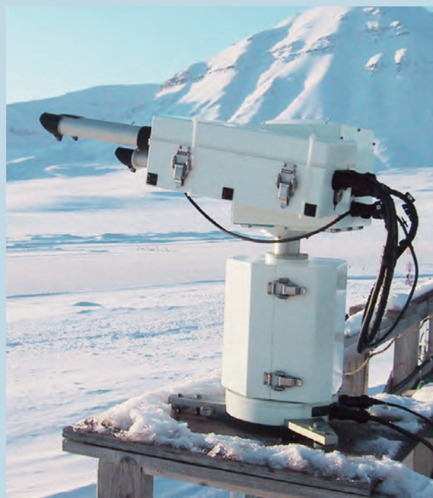
Sky-radiometer for monitoring aerosol optical properties at Ny-Ålesund
