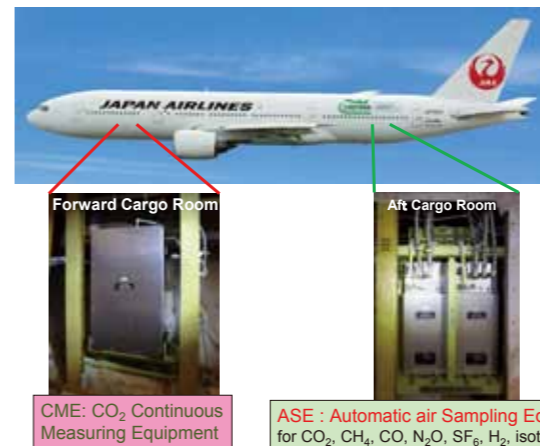
Two types of equipment mounted on a JAL 777-200. They collect samples of air before it is drawn into the jet engine and mixed with air inside the cabin. The day after a flight arrives in Japan, the ASE equipments are sent to NIES for analysis. (Photo credit: Japan Airlines)
