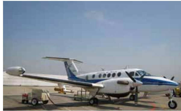
There are only a few special aircraft in Japan that can conduct atmospheric observations. The seats have been removed from the cabin to make room for equipment. There is an inlet on the top of the aircraft to collect aerosols and gases, and there are devices equipped under both wings to measure aerosols, clouds and wind speed. (Photo credit:Koike)
