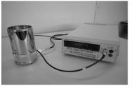
Fig.3 Faraday cage (left) Electrometer (right).
