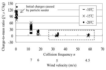
Fig.6 Charge-to-mass ratio Q against the collision frequency n. (Case of spherical particles)
