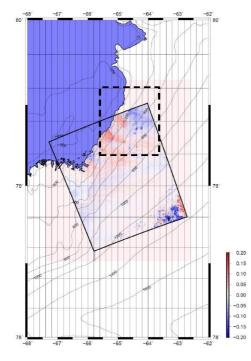
Figure 1. Difference of LOS displacements derived by applying DDInSAR to ALOS/PALSAR data at August 30, October 15 and November 30 in 2007. Unit of scale bar and contor are meter. Bule colar indicates decrease of distance from satellite to surface and red color indicates increase of the distance.
