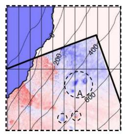
Figure 2. Enlarged image of dashed rectangular region in Fig.1. Spatial size of the largest round-shaped signal in dashed circle A is approximately 2 km and the distance dicrease reaches 15 cm.
