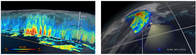
Figure 1. First light of the GPM Core Observatory, observing extratropical cyclone in the northwest Pacific Ocean at 22JST on March 10, 2014. Left: Three dimensional precipitation structure by DPR. Right: Near-surface precipitation by GMI.
