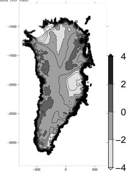
Figure. An example of horizontal distribution of the optimized basal sliding coefficients followind Pollard & DeConto (2012). The ratio relative to the  $I_{C}IES$  default value (3.6 ×  $10^{-10}\,\mathrm{N^{-3}\,yr^{-1}\,m^8}$ ) is shown in the logarithmic scale. The basal sliding parameterization is a Weertman-type formulation with 3rd power.
