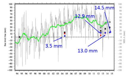
Fig. 2: Change in sea surface height estimated by satellite altimetry and CTD.
