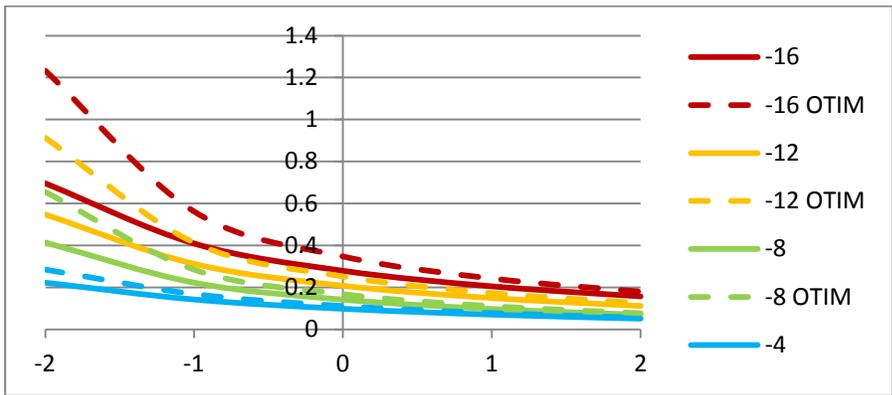
Fig. 1. Thickness versus the difference between surface and air temperatures for different air temperatures
