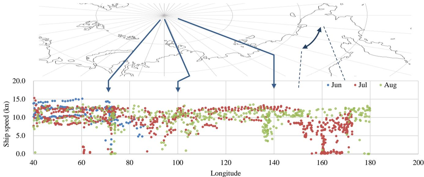
Figure 3. Ship speed distribution along the NSR from Jun. to Aug.
