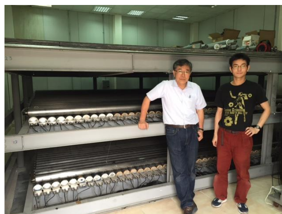
Figure 1. The Kuwait MD with a detection area expanded to 5\text{ m}\times 5\text{ m} . We plan to install similar (but smaller) MD consisting of proportional counter tubes at Syowa station.
