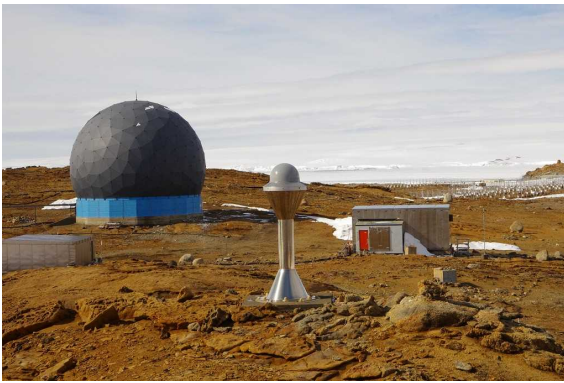
Figure 1. Photo of GNSS antenna (center), gravity measurement room (right), and radome of VLBI antenna (left)
