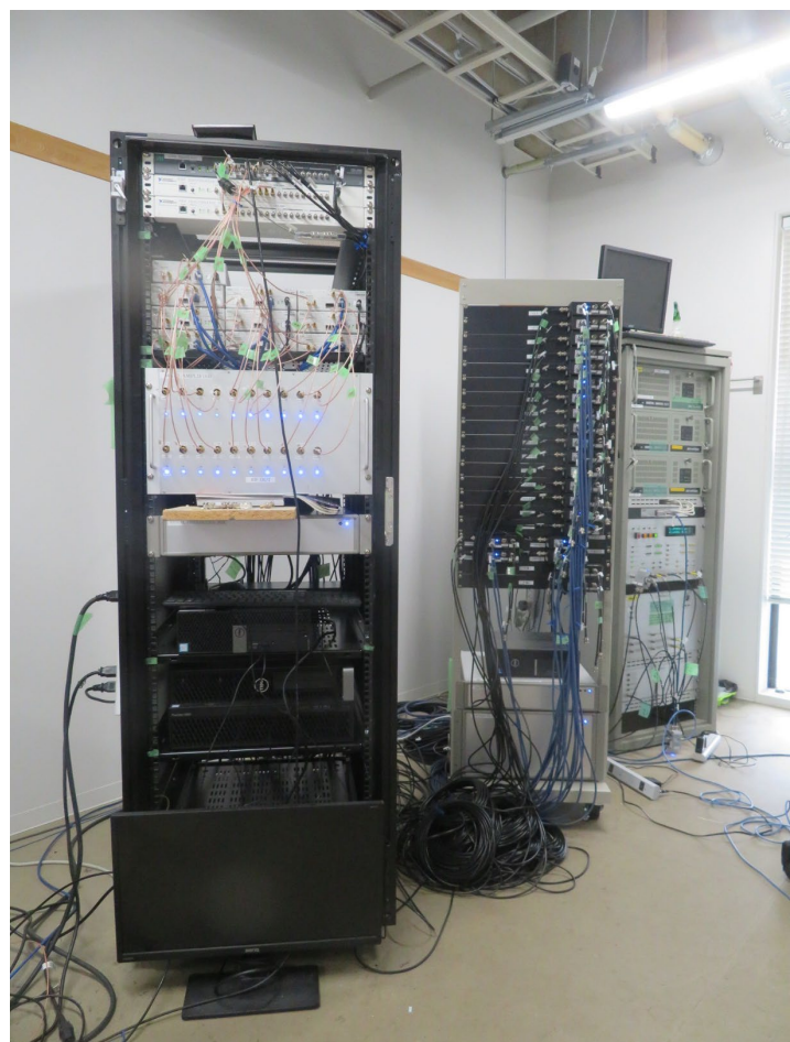
Figure 1. Photo of the main amplifier and control units for the 20-channel imaging receiver system (front), and the head-amplifier (middle). They are now under now under development and to be installed at the SuperDARN Hokkaido East radar site.
