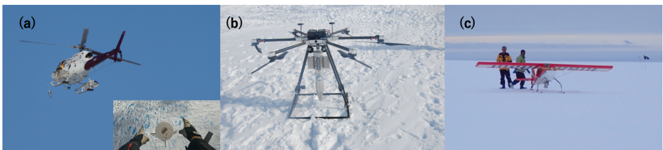
Figure 1. (a) The penetrator dropped from an AS350 helicopter and penetration installation observed from the air, (b) Drone with penetrator at S16 (left), and (c) UAV just before takeoff test at the S17 site
